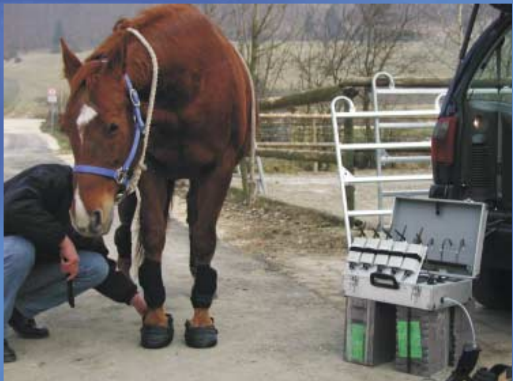
Computer Kinematography (CKG): Wireless technology is used to transmit data from sensors in the bandages to an advanced computer system.
